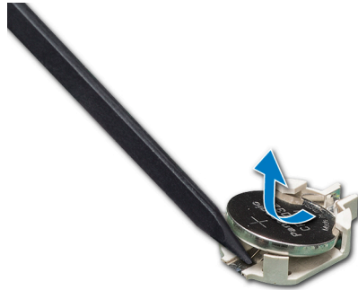
Figure 108. Removing the system battery
