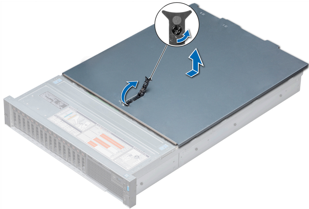
Figure 19. Removing the system cover
