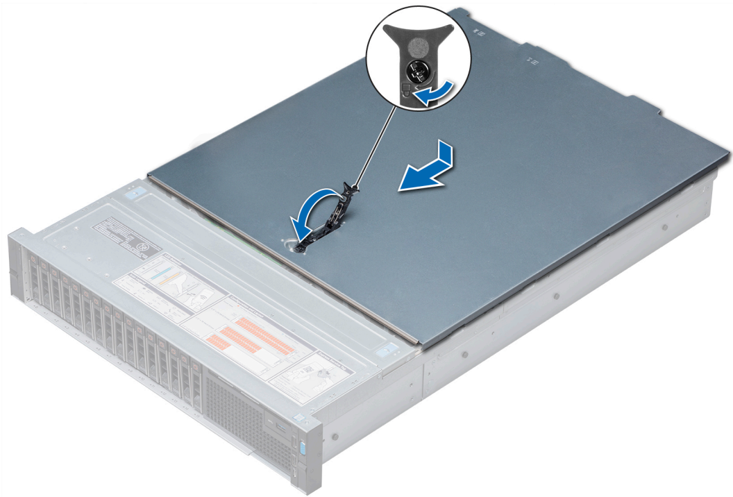
Figure 20. Installing system cover
