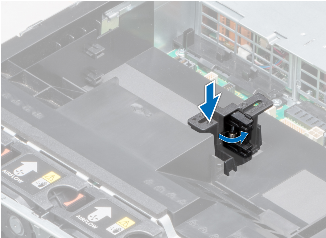
Figure 55. Opening the PCIe card holder latch
